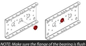
against the sheet metal of the gearbox plate.
