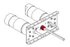
**Step 6**: Install one Gear Assemblies onto the center axle of the gearbox. Be sure to place the boss of the Gear against the spacer. Tighten the #10-32 set screw to lock the Gear Assembly in place.
