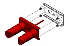
**<u>Step 10</u>**: Secure the gearbox together with four 1/4-20 Nylock Jam Nuts (am-1102)
