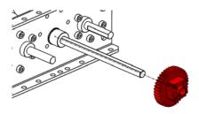
**Step 7**: Install a Gear Assembly onto each of the NeveRest Motor shafts such that all of the gears in the Gear Assemblies are lined up. Tighten the #10-32 Set screws to lock all the gear assemblies in place.
