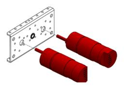
**Step 3**: Install six M3-0.5 x 6mm long socket head screws (am-1254) in each NeveRest motor to secure it to the gearbox plate.
